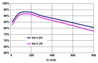
FIGURE 3. EFFICIENCY (Vin = 3.6V)
