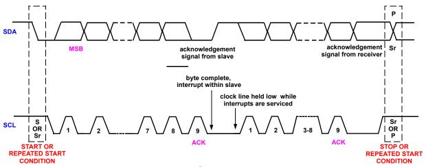
FIGURE 17. I<sup>2</sup>C DATA AND CLOCK
