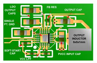
FIGURE 27. COMPONENT PLACEMENT AND TOP COPPER
