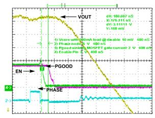
PGOOD delay = 186ns from disable. Vout = 0.85V prior to EN going low, 400ns/DIV
