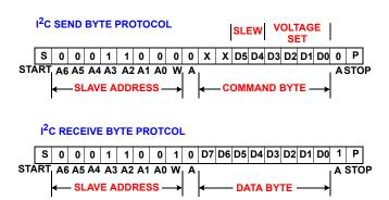
FIGURE 18. INTERFACE BIT DEFINITION AND PROTOCOL
