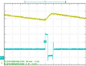
Ripple in DCM: Fripple = 145kHz, Vin = 2.85V, Vout = 0.85V, lout = 10mA Ripple = 10mV (worst case), 1µs/DIV
