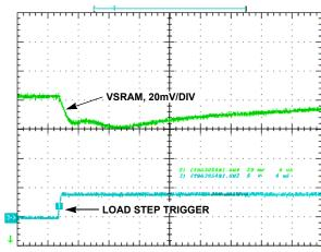
LDO transient response with 3.3µF output capacitance. LVCC = 4.1V. 10mA DC load+ 55mA step load.
