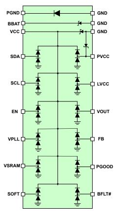
FIGURE 26. INTERNAL ESD STRUCTURES
