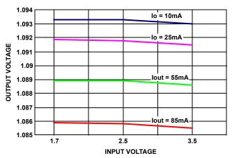
FIGURE 4. VSRAM LINE-LOAD REGULATION
