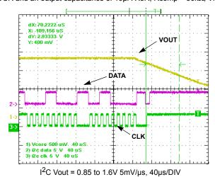
FIGURE 8. TYPICAL I<sup>2</sup>C COMMUNICATION
