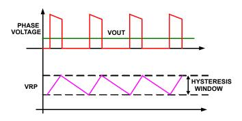
FIGURE 21. SYNTHETIC RIPPLE REGULATION IN CCM
