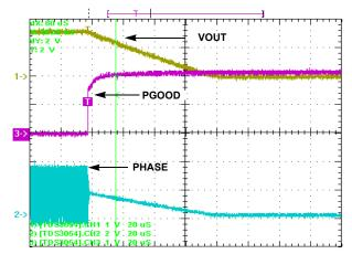
Forced PGOOD fault. Converter operating in CCM at 420mA prior to applying a 320mA transient step. This pushes the regulator beyond the overcurrent threshold of 700mA. The phase node three-stated and follows Vout to 0V. 20µs/DIV
