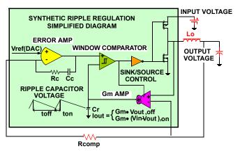
FIGURE 20. SIMPLIFIED SRR DIAGRAM
